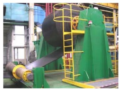
The machine is composed of two reeling machines (Figure 4), two pushing devices, a maintenance table and two series-connected guiders to guide the strip onto the reels.
